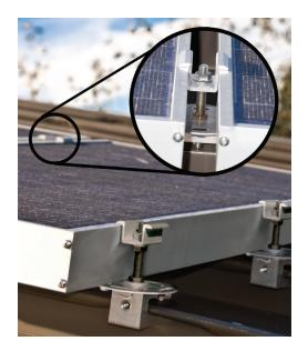
The challenge has been in how to attach the PV modules to the standing seam roof systems without jeopardizing roof material and weather-tightness warranties. The answer is the S-5-PV Kit and the S-5! Mini.
