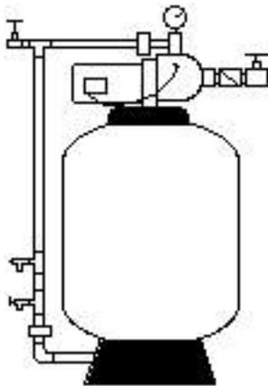
A typical pressure booster system consists of a jet pump, hydropneumatic tank, pressure switch, and check valve. When demand occurs, the pressure switch senses a pressure drop and starts the pump. When demand disappears, the pump continues to run until the tank is filled and pressure reaches shut off level. A check valve on the suction side of the pump prohibits the pressurized water
