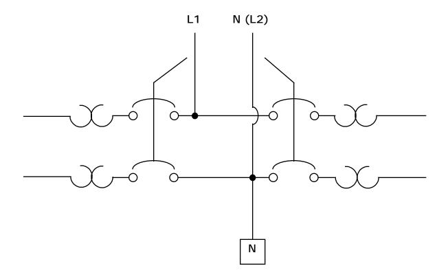
CE21SW AND CE21DW CONTROL PANELS ARE WELL SUITED FOR 115 VAC INSTALLATION. FOLLOW THE DIAGRAM ABOVE AND STEPS BELOW WHEN WIRING FOR 115 VAC.
