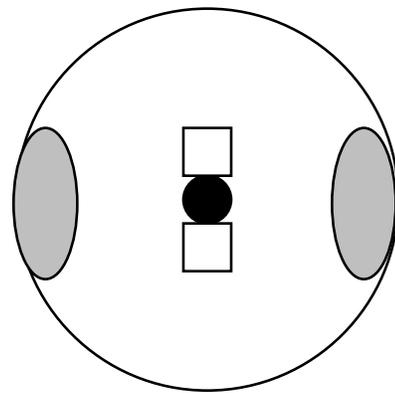
Since our electric current changes direction 60 times per second our 2 pole motor's synchronous speed will be 3600 rotations (not revolutions) per minute (RPM). The full load speed (or slip speed) will be somewhat less, usually between 95 and 99% of synchronous speed.
