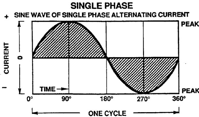
During one 360 degree cycle of AC, current is 0 at 0 degrees, +max at 90 degrees, 0 again at 180 degrees, -max at 270 degrees, and finally 0 at 360 degrees. Current varies at every point in between. In the US this cycle occurs 60 times each second. In Europe and some other countries it is reduced to 50.
