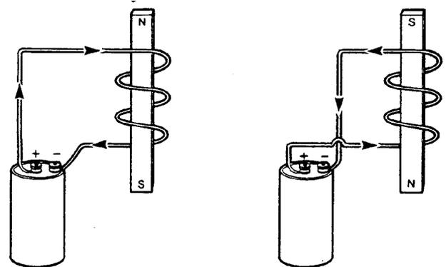
This ability to change polarity is the basis for the simple DC motor that many of us built in elementary school. On the following page, we see a loop of wire (rotor) within a permanent magnetic field (stator) and connected to a battery via contacts that change current direction every half rotation (commutator). When current passes through the loop, it flows in one direction in the upper half and in the opposite direction in the
