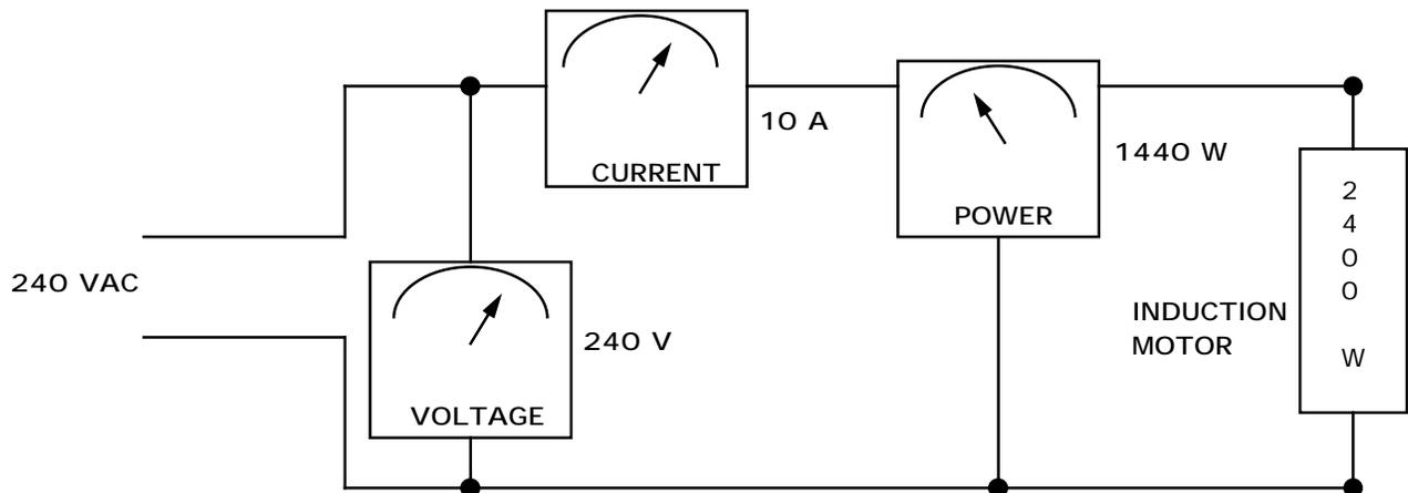
Both of the circuits above are powering 2400 watt loads. The volt and amp meters in both read 240 volts and 10 amps respectively. Although the motor is at nearly full load, its watt meter is indicating far less power consumption than the watt meter in the water heater circuit. Do both of these circuits obey Ohm's law? Is not a watt a volt amp? Explain what is going on here and suggest a method of fixing this obvious discrepancy.
