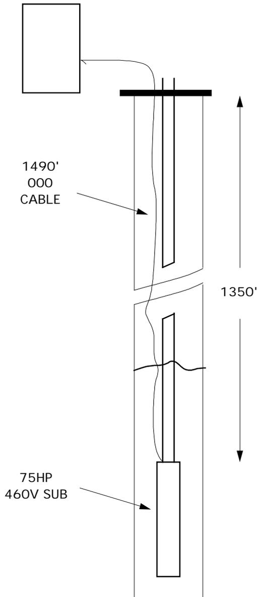
ONE OF OUR BIG ISLAND CUSTOMERS PLANS TO INSTALL A 75HP, 460V SUBMERSIBLE AT A SET DEPTH OF 1350'. THE LOCAL UTILITY SAYS THAT THEY REQUIRE REDUCED VOLTAGE STARTING ON MOTORS OF THIS SIZE DUE TO THE EXISTING ELECTRICAL LOAD IN HIS RUAL AREA. THEIR REQUIREMENT CALLS FOR A 30 - 35% REDUCTION IN THE NORMAL STARTING CURRENT. OUR CUSTOMER CLAIMS THAT HIS PUMP WILL MEET THEIR REQUIREMENTS WITHOUT ANY ADDITIONAL STARTING HARDWARE. THE UTILITY OFFICALS DISAGREE. WHO IS RIGHT AND WHY?
