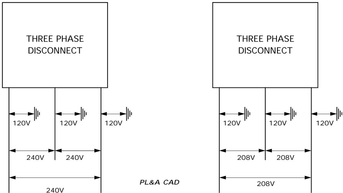
A mechanical contractor ran into the situation shown above while he was replacing some booster pumps in a large Waikiki hotel. In one of the older buildings the three phase supply voltage was 240V. In a newer section, however, he found the supply voltage to be 208V. In both areas all legs read 120V when measured to ground. Why does the supply on the right read 208V leg to leg? Are not the legs additive? How can  $120 + 120 = 208$ ?
