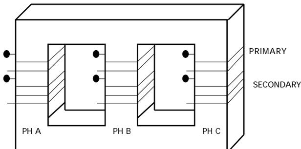
Again, like the ac motor stator, the primary and secondary windings of a transformer may be either delta and wye connected.
