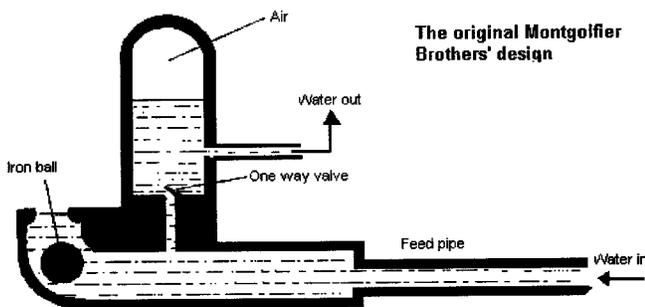
Water enters the Ram from the supply or "drive" pipe, flows through it, and discharges through the upturned end on the left. Inside
