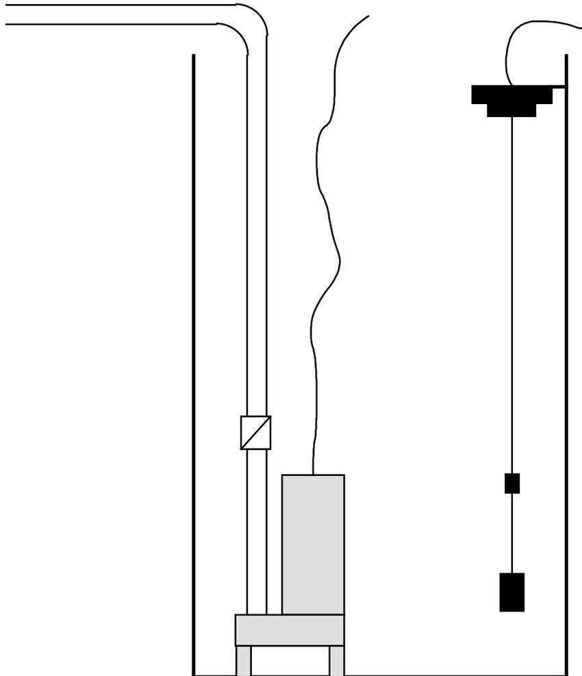
The sump pump shown above is pumping up a short rise to a 4" gravity main that services several homes. On occasion, the pump will air lock and has to be manually primed before it will pump again. A single, wide angle float switch controls the pump. In the off (down) position the float, and therefore the water level, is well above the pump's discharge. If the float is shutting the pump off at the proper level, what could be causing it to air lock?
