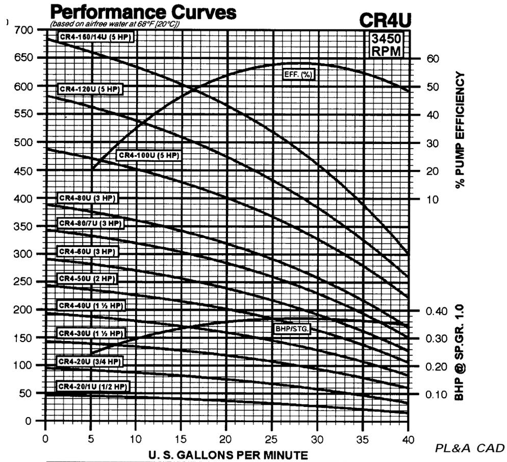
One of our food processing customers wants to purchase a washdown pump that will deliver between 25 and 30 gpm. He has deduced upon the CR4-160/14U which is a 5hp, 14 stage unit (upper curve above). His plant power is 208V, 3 phase. We have the pump and a tri-voltage, 5hp motor in stock. Should we sell him this combination or should we order a 5hp motor designed specifically for 208V? Are there any other options available?
