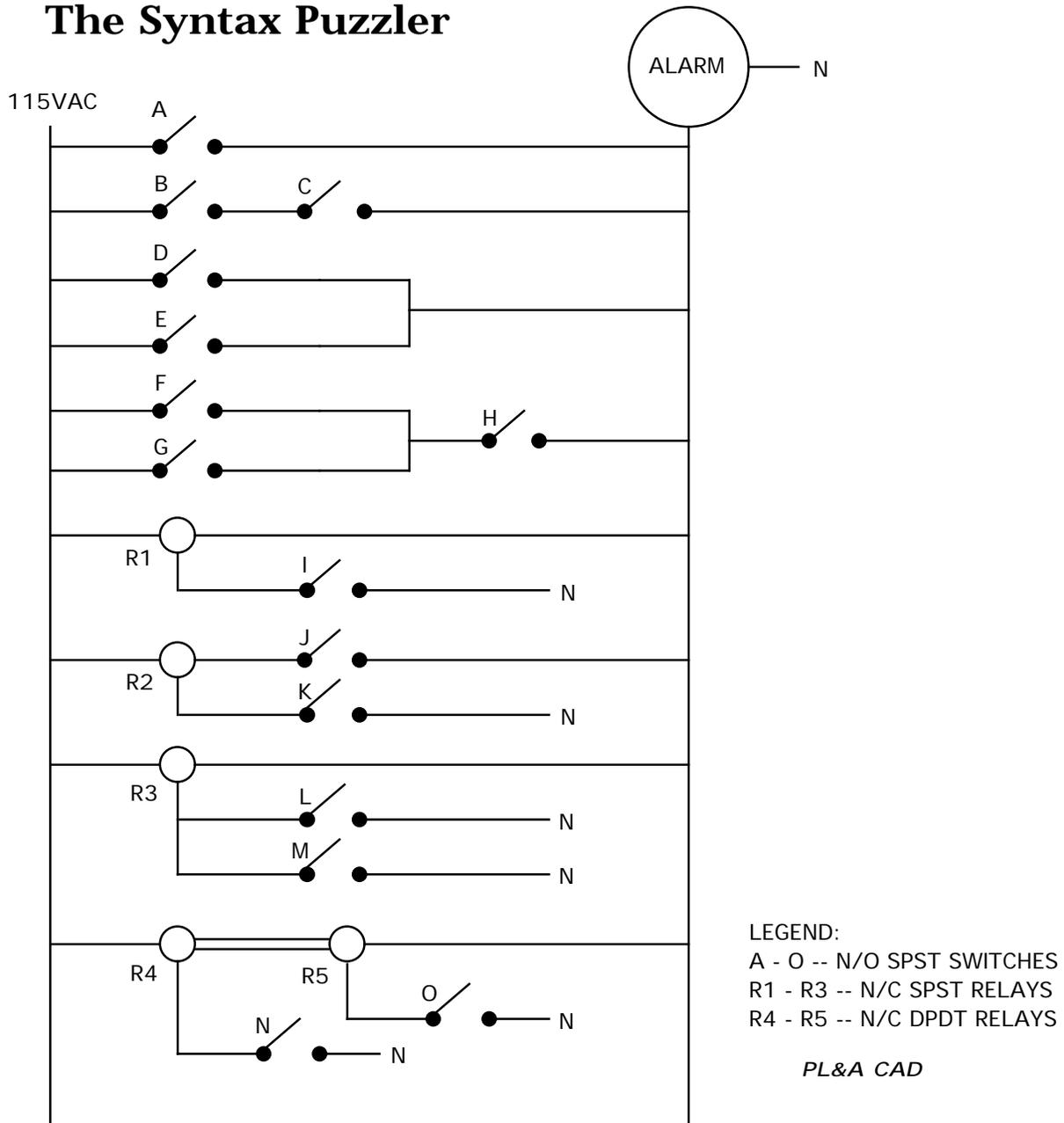
The schematic diagram shown above is that of an alarm circuit. It was designed by a somewhat overly cautious engineer. (Is there a hyphen in anal retentive?) Please list the conditions that will cause an alarm.
