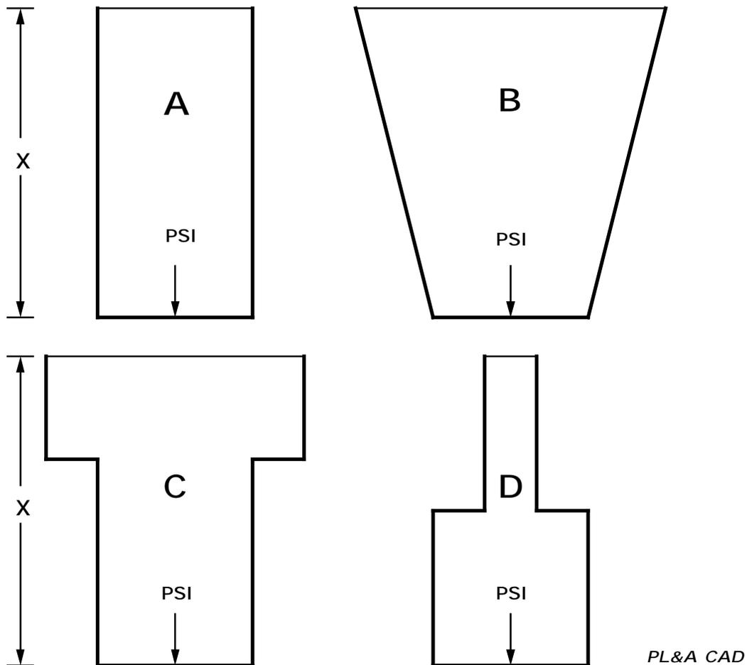
The height of the liquid ( $x$ ) in each of the containers is the same. The area of the base of each container is also equal. The pressure (in psi) exerted on the bottom of each container is also the same. How can this be if their volumes (and therefore the weights of the liquid) vary considerably?
