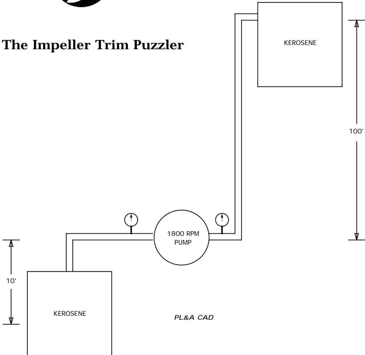
An underground tank supplies kerosene to a centrifugal pump at ground level. The pump, in turn, supplies another tank that is 100 feet above its discharge. Ignoring friction within the system, what diameter must the pump's impeller be if it is rotating at 1800 rpm? Also what pressure will be indicated by the two gauges?
