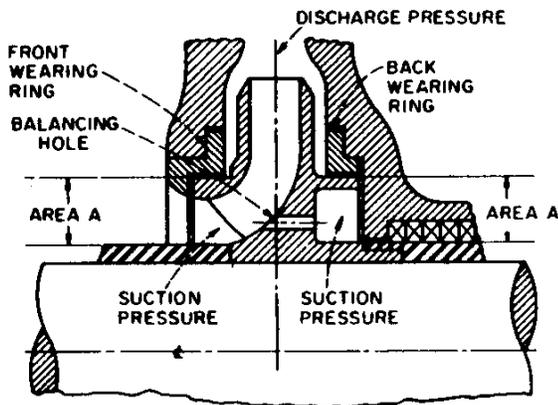
By incorporating a wear ring and balancing holes in the back shroud, the surface area is reduced by an amount equal to the impeller eye. Since that portion is now under suction pressure, the volute axial forces are nearly equal and axial thrust is greatly reduced.
