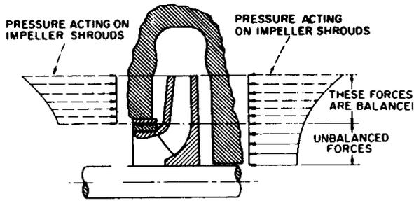
In the case of the overhung impeller (typical end suction pump) increased suction pressure decreases axial thrust while suction lift increases it. In small pumps this axial thrust can easily be accommodated by the pump or motor bearings assuming they are sized correctly. With very large pumps or those under extremely high suction pressure, this increased axial thrust can be significant and must be considered during design.
