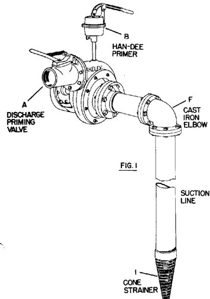
The hand operated diaphragm pump (B) removes air from the pump case and suction piping while atmospheric pressure forces water into the evacuated space. A check
