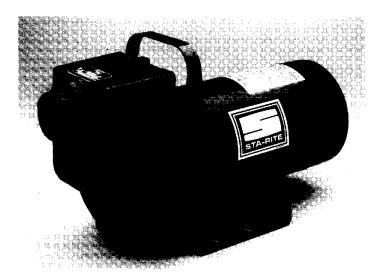
The DPC self-priming centrifugal pump is a rugged cast iron pump capable of priming up to 20' vertically. The semi-open impeller will handle solids up to .225". The unit is equipped with a 1/2 HP 115 volt motor and features 1-1/4" suction and discharge.
